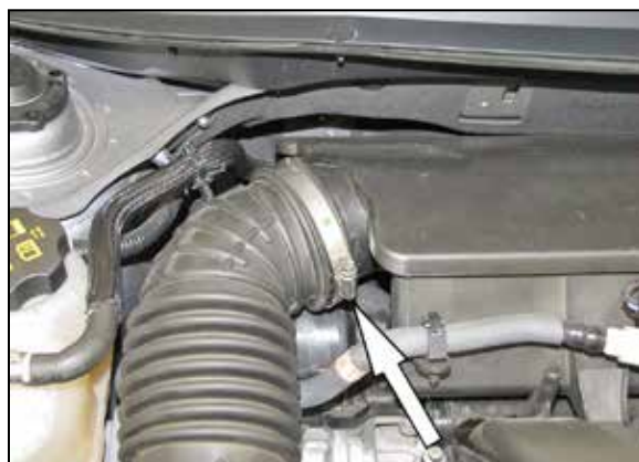
4. Loosen the hose clamp that secures the intake tube to the intake plenum.
