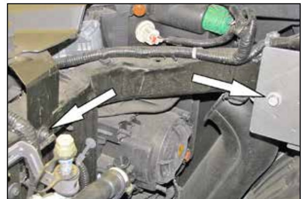
6. Remove the two factory bolts shown. NOTE: These bolts will be reused in a later step.
