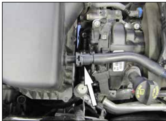
3. Disconnect the crank case vent hose from the air filter housing.
